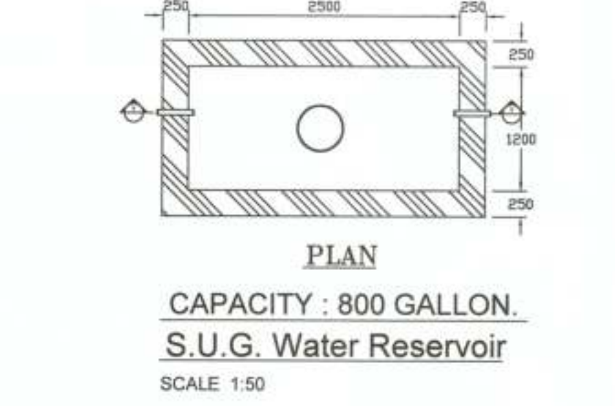
PLAN CAPACITY : 800 GALLON. S.U.G. Water Reservoir SCALE: 1:50
